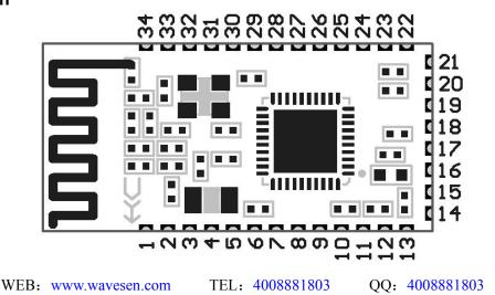
The HC-08 module has 34 pins, on board PCB antenna, pin specific definitions are listed in the following table:
