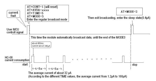
The user MCU to the module of UART port to send 10 bytes hexadecimal code of "0xFF, 0xFF, 0xFF,
